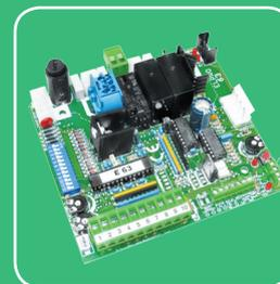
Incorporated electronic control board ELPRO 63, pre-set to take the plug-in radio receiver
