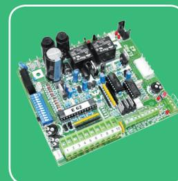
Incorporated electronic control board ELPRO 62, pre-set to take the plug-in radio receiver
