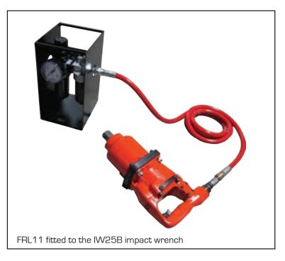
We strongly advise to use this FRL11 unit with all air operated tools and air driven pumps, such as IW series of pneumatic impact wrenches (see page 91), the AHP11 series foot operated air driven pumps (see page 46 to 47) and similar air driven tools, to maintain integrity of air supply.
