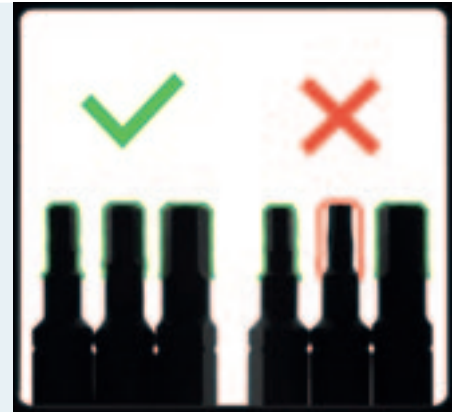
Bit detection using a backlight
