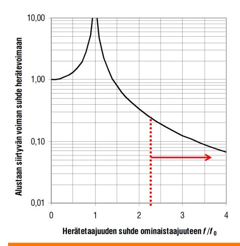
f = lowest characteristic frequency of the equipment to be isolated (e.g. the rotation speed/frequency of fan)
