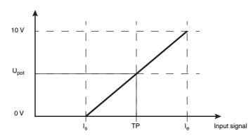
$\begin{array}{ll} I_{\rm s} = & & {\rm Starting\ point} \\ TP = & & {\rm Trip\ point} \\ I_{\rm e} = & & {\rm End\ point} \\ U_{\rm pot} = & & {\rm Proportional\ switching\ voltage} \end{array}$
