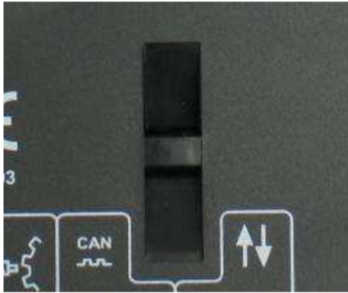
Cable Tie Fixing Point
