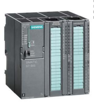
SIMATIC S7-300, CPU 313C, COMPACT CPU WITH MPI, 24 DI/16 DO, 4AI, 2AO 1 PT100, 3 FAST COUNTERS (30 KHZ), INTEGRATED 24V DC POWER SUPPLY, 128 KBYTE WORKING MEMORY, FRONT CONNECTOR (2 X 40PIN) AND MICRO MEMORY CARD REQUIRED
