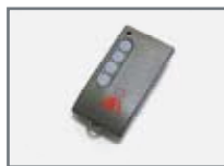
D111300 - T03D Transmitter with triple coding with four buttons for 3 codes. The first 3 buttons send a signal using 3 codes while the fourth button uses the third code with another channel. Useful in small apartment blocks with two gates in common and a private overhead door. Available while stock last.
