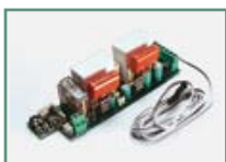
D113050 - SPL Preheating board for 1 or 2 LUX, SUB, ORO, P4,5-P7, BERMA and E5 operator models. With this accessory the
