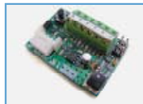
P125005 - BT BAT Thanks to the back-up batteries and battery charger, the BT BAT kit guarantees low voltage operation of the leaf in the event of power failure (LIBRA C MA, LIBRA C LX, HYDRA R).
