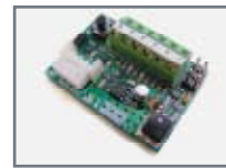
P111408 - SCS WIE Circuit board for direct connection of wiegand accessories (such as SELETTTO, COMPAS SLIM, etc) to the control units QSC D MA, LIBRA C MA, LIBRA C MV, LIBRA C LX, VENERE D, LEO D MA, LEO MV, RIGEL 5 and ALTAIR P.
