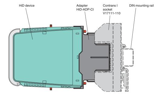
Connection assignment of the adapter as interface between HiD device and V17111-110 Contrans I socket
