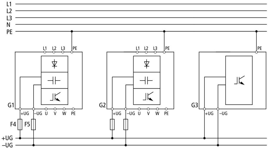
Figure 17: DC main feed with interconnected DC bus
