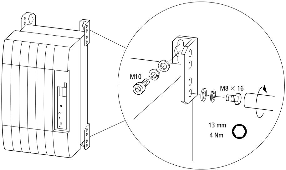
Figure 42: Fixing to the mounting plate
