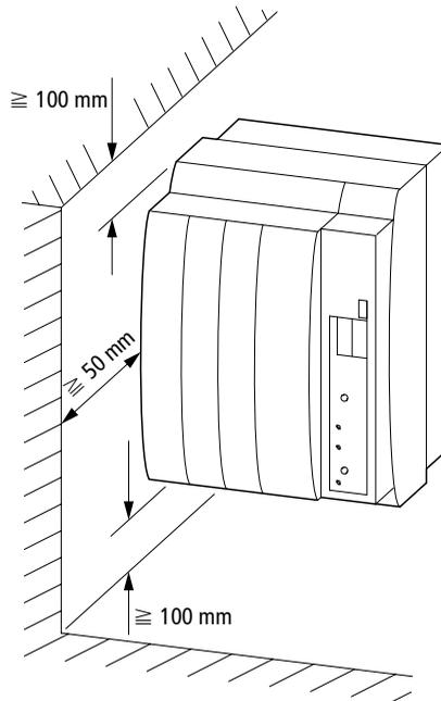
Figure 37: Necessary clearances for the DF4 series
