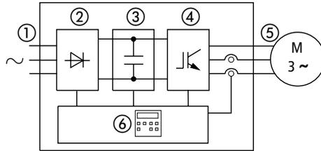
Figure 3: Block diagram of a frequency inverter
