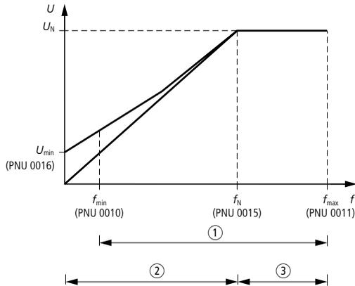
Figure 33: Usable motor speed range
