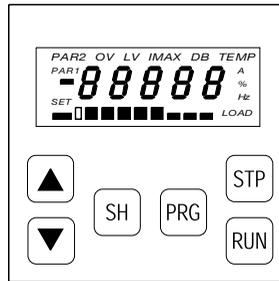
Figure 47: Display symbols on the LCD keypad
