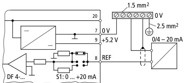
Figure 26: Analog setpoint with current loop signal
