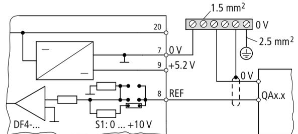
Figure 24: Setpoint entry from a PLC
