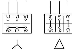
Figure 6: Circuit configuration
