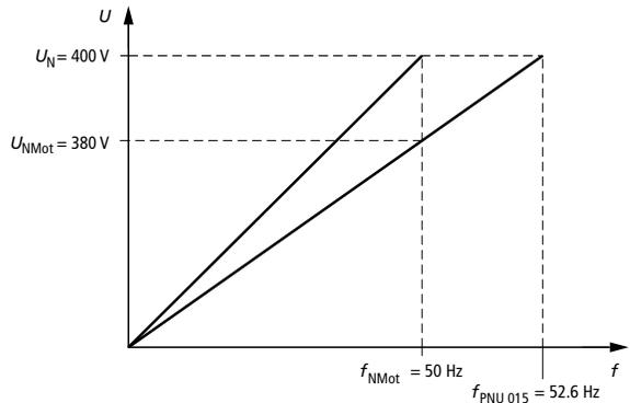
Figure 32: Calculation of characteristic point PNU 015
