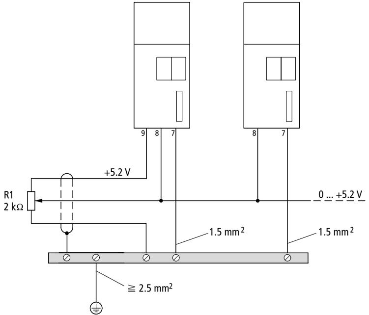
Figure 25: Master setpoint signal for several frequency inverters
