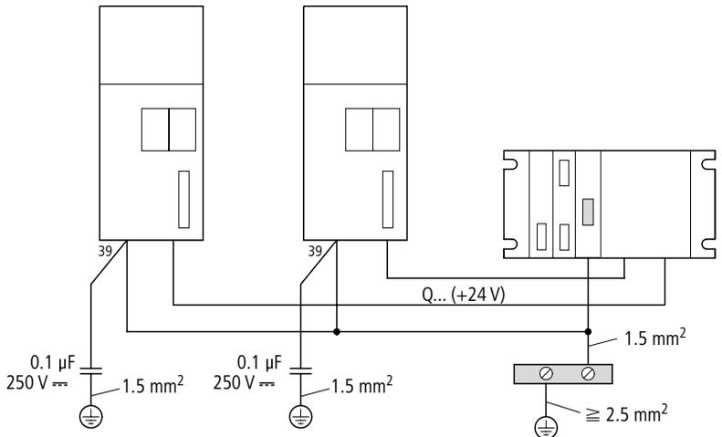
Figure 22: Earthing when a PLC is used
