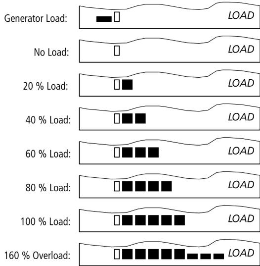
Figure 48: Motor load display
