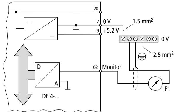
Figure 28: Connecting a meter to the monitor signal
