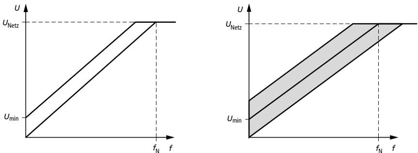
Figure 31: Constant and automatic motor voltage boost
