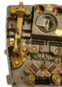
1976 Digital Mass Transducer MK-I with two vibrating wires
