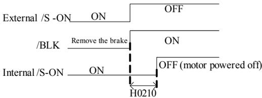
**【Note】** The servomotor will turn OFF immediately when a fault occurs, regardless of the setting of this parameter. The movable part of the machine may shift due to gravity or external force before the brake operates.
