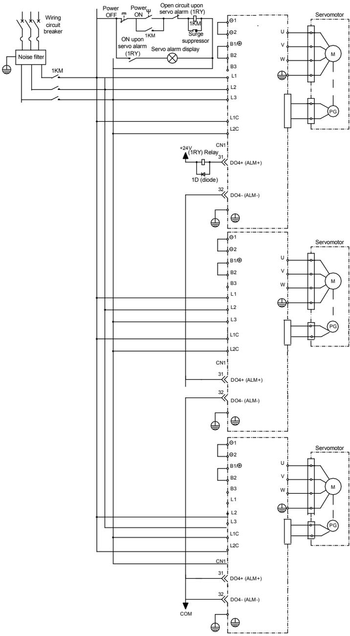
Multi-drive Wiring (Alarm Output Signal is Normally Open Terminal)
