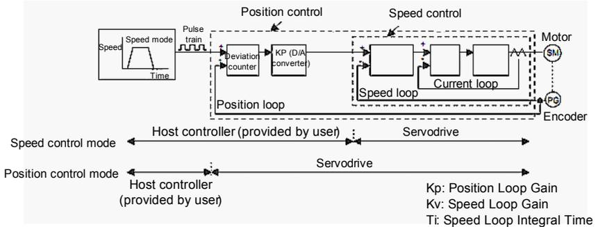
In general, the position loop response cannot be higher than the speed loop's. Therefore, to increase the position loop gain, increase the speed loop gain first. If only the position loop gain is increased, speed reference vibration may result, finally extending the positioning time.
