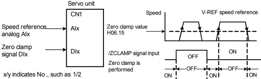
If vibration occurs when zero-position fixed function is enabled, you can set the position-loop gain through H08-02. If the 2nd gain switching function is enabled, 2nd Position-loop Gain (H08-05) also needs to be adjusted.
