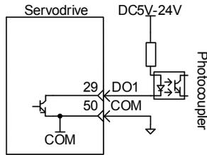
Maximum allowable voltage/current of Servodrive internal photocoupler output circuit is as follows:
