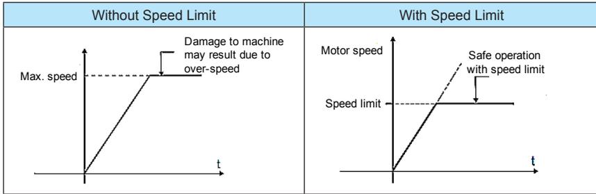
Signals output during servomotor speed limit is shown as follows:
