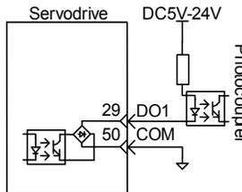
Maximum allowable voltage/current of servodrive internal photocoupler output circuit is as follows:
