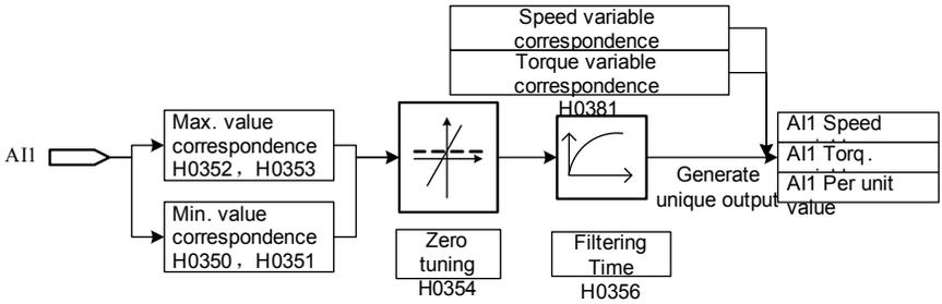
Designate analog using method based on the function codes below .
