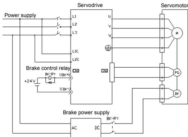
The brake signal output is shown as below:
