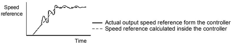
In general, the position loop gain cannot exceed the mechanical system natural vibration frequency range. For example, multi-joint robot's overall structure has low rigidity since it uses volatile gear reducer. Its natural vibration frequency is 10-20Hz. So the position loop gain of such machine is 10-20Hz only.
