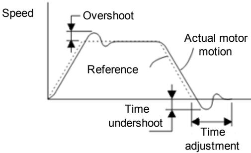
The mode switch function automatically switches the speed control mode from PI control mode to P control based on a comparison between the servo’s internal values.
