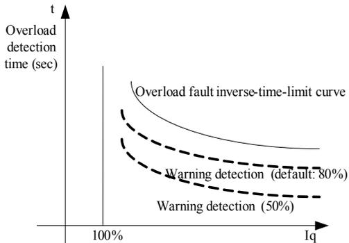
The following table lists the overload feature of the servomotor.
