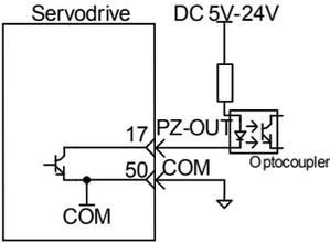
Maximum allowable voltage/current of the servodrive internal photocoupler output circuit is as follows:
