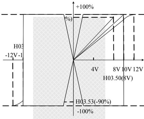
In the above figure, the shaded areas can realize full scale  $\pm 100\%$  at any voltage. In other areas, full scale cannot be realized or the analog voltage precision cannot be fully utilized.
