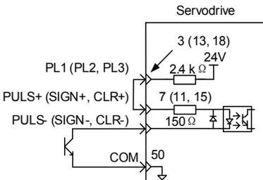
When external power supply is used, the circuit is as follows:
