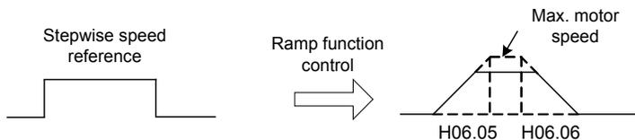
The acceleration/deceleration slope time is determined by the time the motor takes from 0 to maximum speed (or from maximum speed to 0). The actual acceleration/deceleration slope time is calculated as below:
