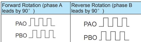
If the encoder feedback pulse output signal is not in the same direction as the host controller reference, you can adjust rotation direction (H02-02) or output feedback direction (H02-03).
