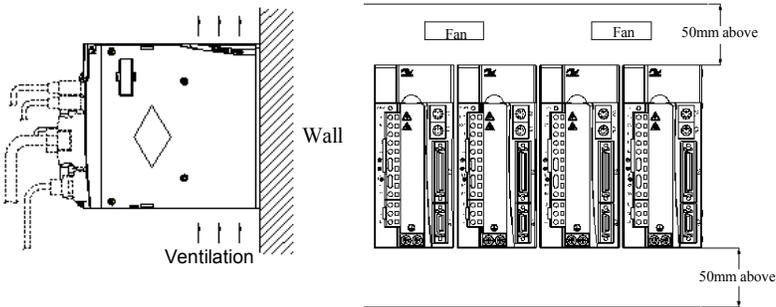
Install the servodrive perpendicular to the wall and make the front panel of the servodrive face outward.
