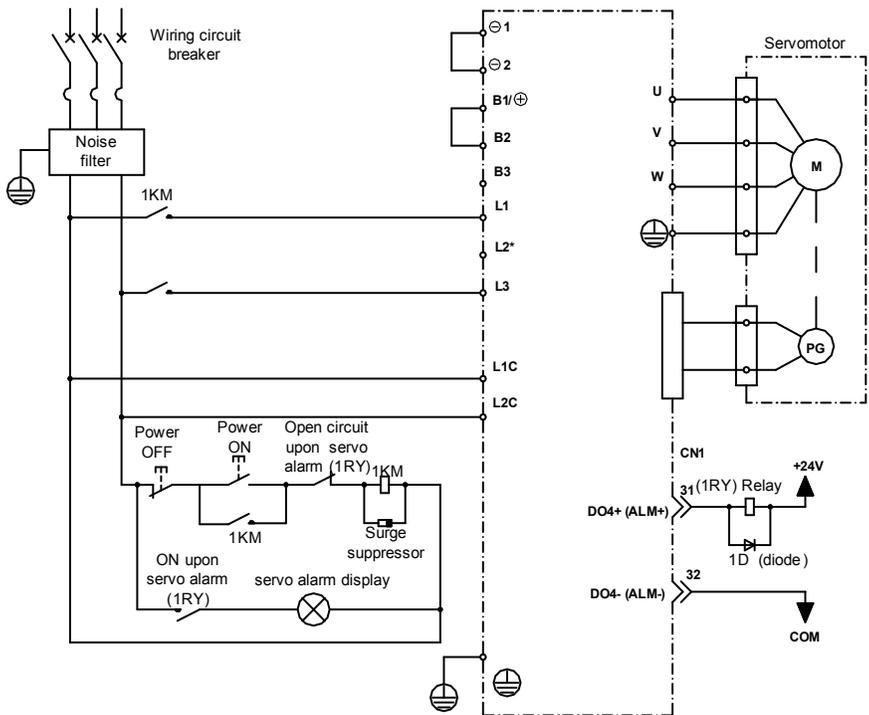
**[Note]** In the single-phase 220V wiring, servodrive does not use L2. Thus, wiring L2 is prohibited.
