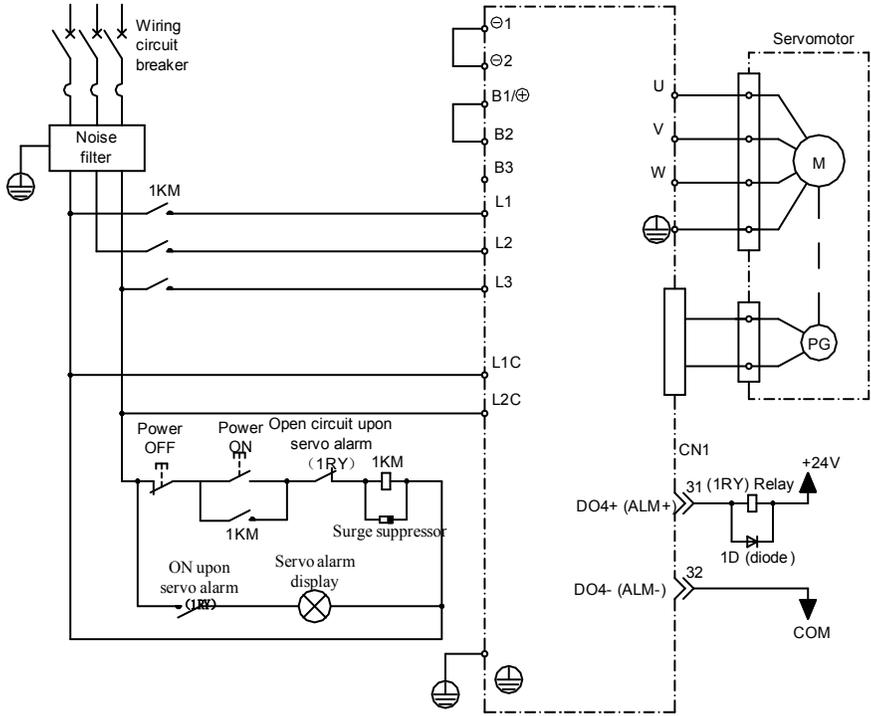
■ Multi-drive Wiring (Alarm Output Signal is Normally Closed Terminal)
