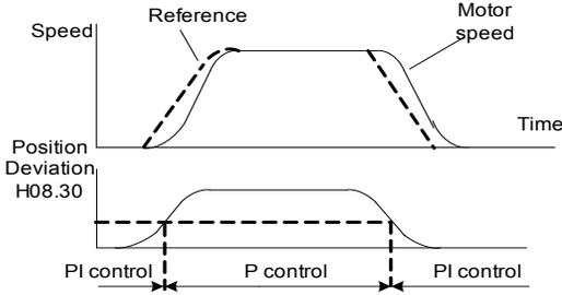
It is necessary to increase the speed loop gain to reduce the adjustment time, resulting in overshooting or undershooting, which can be suppressed by using the mode switch via position error pulse.
