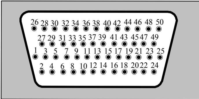
5.3.3 I/O Signal (CN1) Names and Functions
