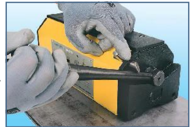
Use of the 2 hands necessary during deactivation
