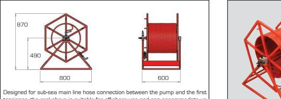
Designed for sub-sea main line hose connection between the pump and the first tensioner, the reel above is suitable for off-shore use and can accommodate up to 300 meters of Hi-Force XHC hydraulic hose. The reel comes complete with quick connect couplings, integrated brake and a spring loaded locking bolt.
