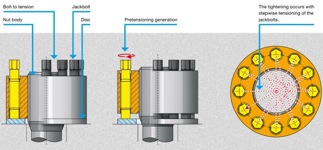
After the pretensioning force generation, the MSN stays on the bolted respectively component connection. Due to mounting without further accessories, the MSN is an economic and effective axial bolt tensioner with little diffusion.
