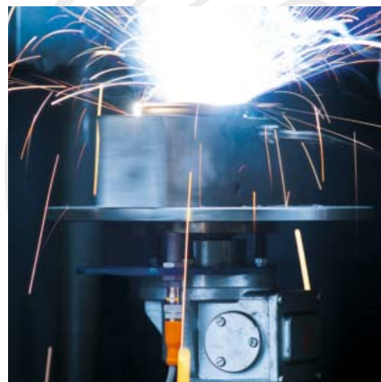
ecolink EVW – thanks to a non-stick coating resistant to weld spatter.
