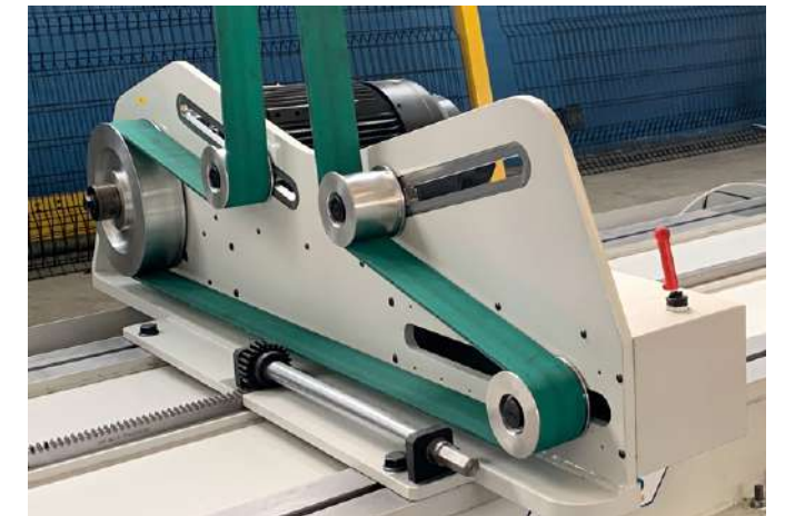
Belt drive system with pneumatic tensioning tool. Belt drive systems are also available with manual arm tensioning tool.
