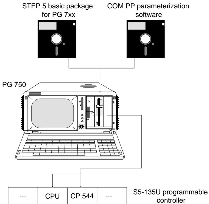
Fig. 9-2 Use of programmer for point-to-point link
