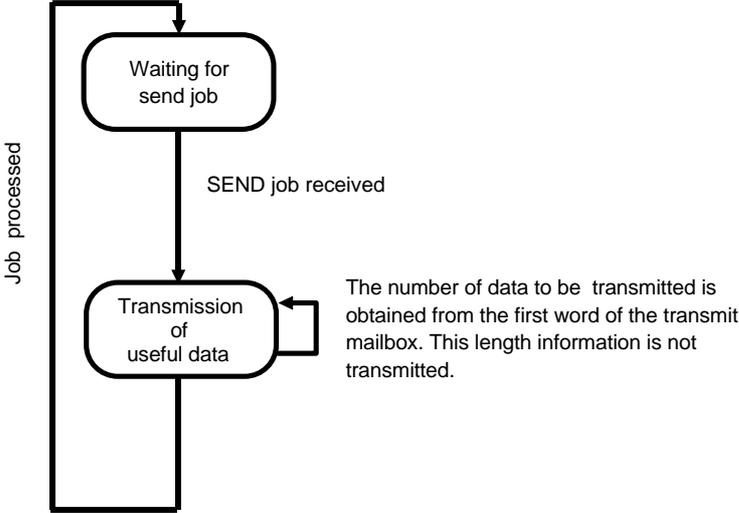
Fig. 5-8 Transmission sequence in mode 3
