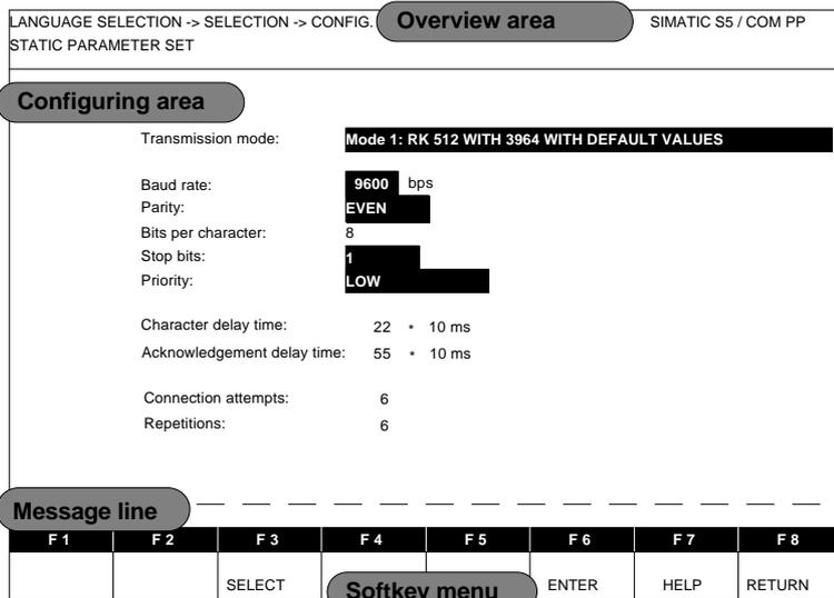
Fig. 7-2 Layout of a screen form
