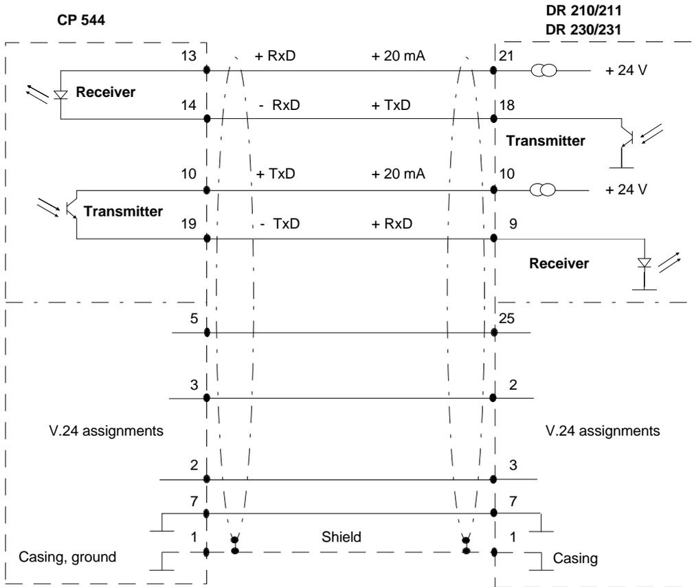
Fig. 10-5 TTY submodule: connecting cable CP 544 - DR 210/211, DR 230/231
