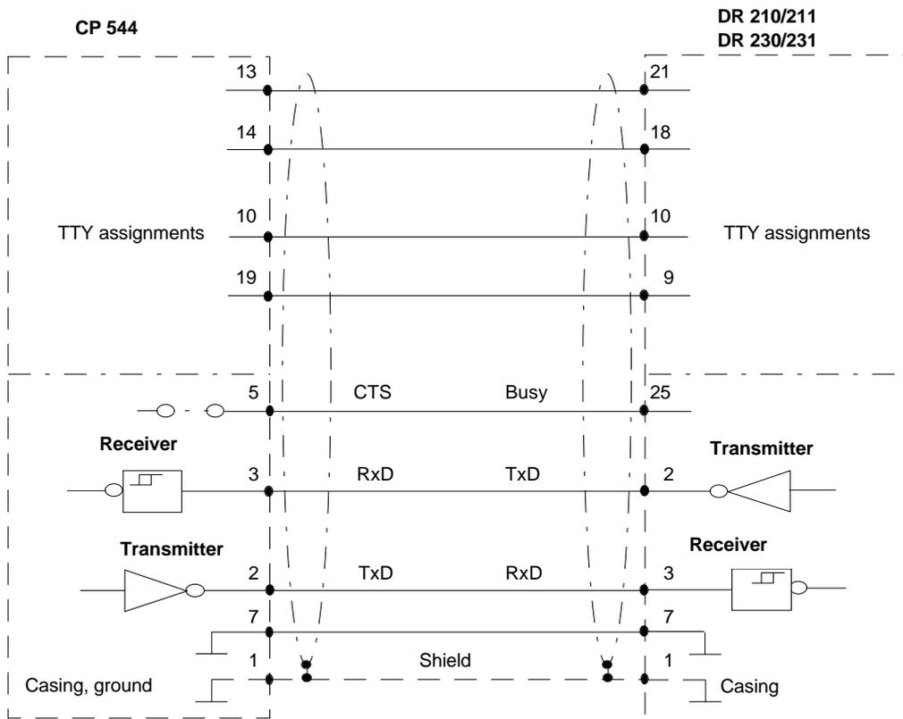
Fig. 10-10 V.24 submodule: connecting cable CP 544 - DR 210/211, DR 230/231
