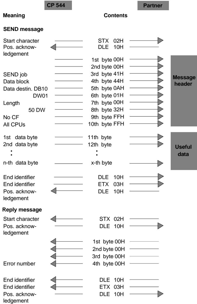
Fig. 3-10 Sequence of a SEND message with reply message
