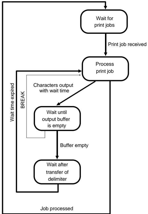
Fig. 5-10 Transmission sequence in mode 4
