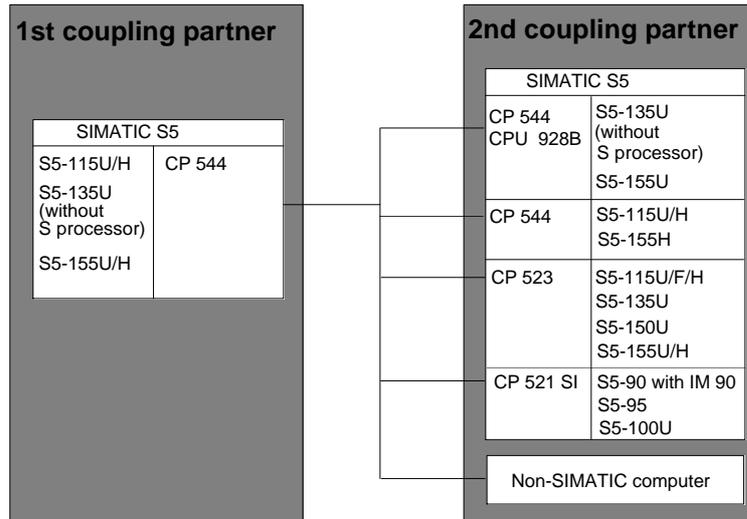
Fig. 4-1 Possible coupling partners for data transmission with the 3964/3964R procedures
