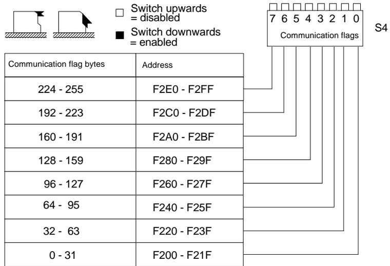
You must additionally enter the corresponding coordination flag bytes in the DB1 of the CPUs! They can then be addressed in the STEP 5 program.
