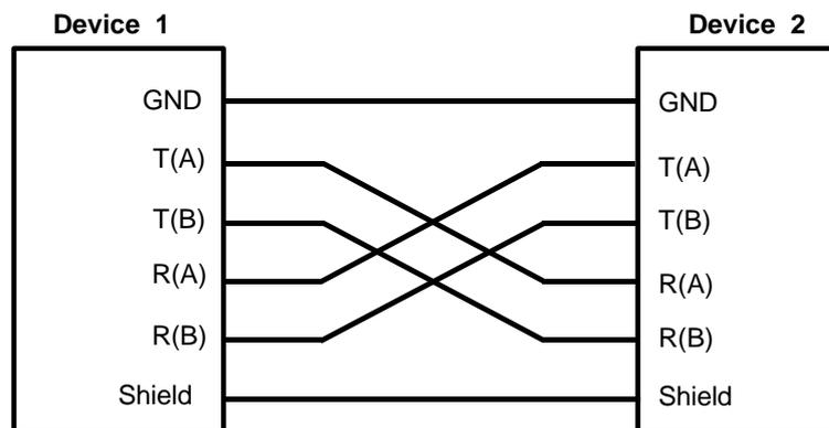
Fig. 1-3 RS422/485 submodule: full-duplex mode
