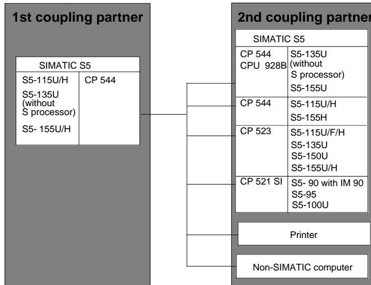
Fig. 5-1 Possible coupling partners for data transmission with open driver
