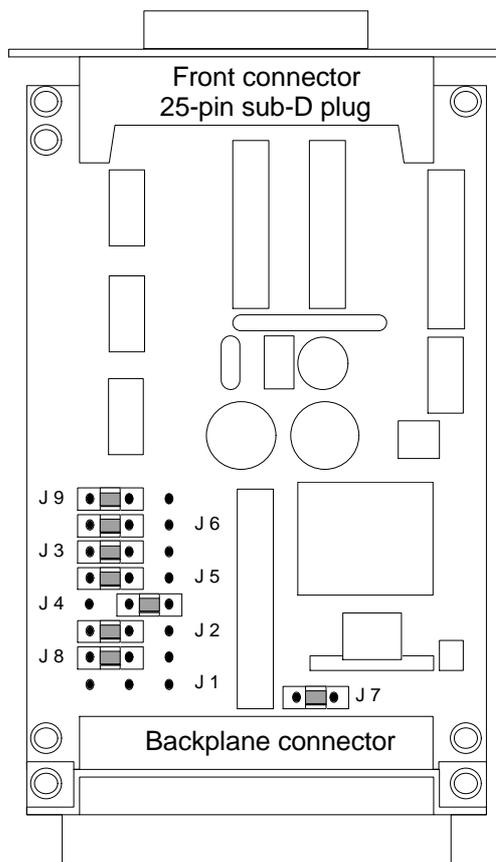
Fig. 10-8 V.24 submodule: jumper settings when supplied
