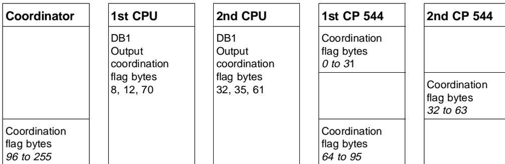
The first CPU is to coordinate the data transfer with the first CP 544 via the bits of the coordination flag bytes 8, 12 and 70.
