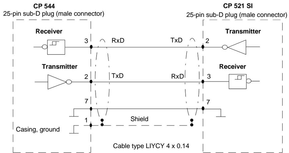
Fig. 10-12 V.24 submodule: connecting cable CP 544 - CP 321 SI
