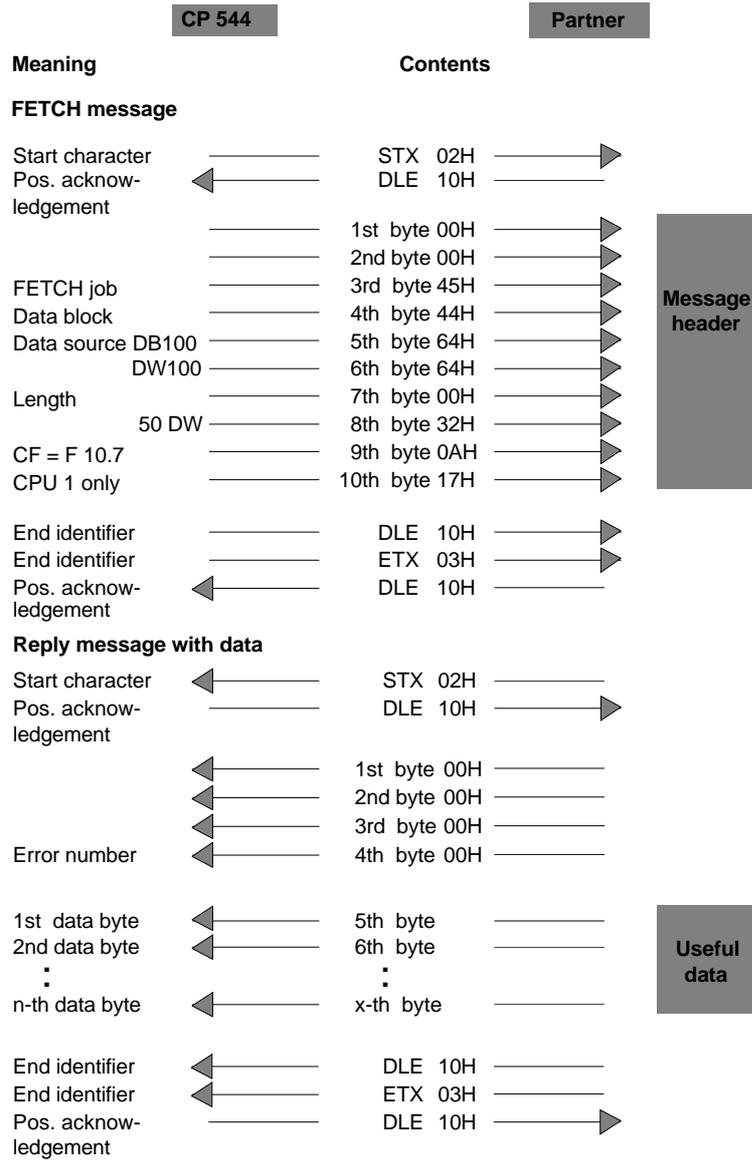
Fig. 3-13 Sequence of a FETCH message with reply message
