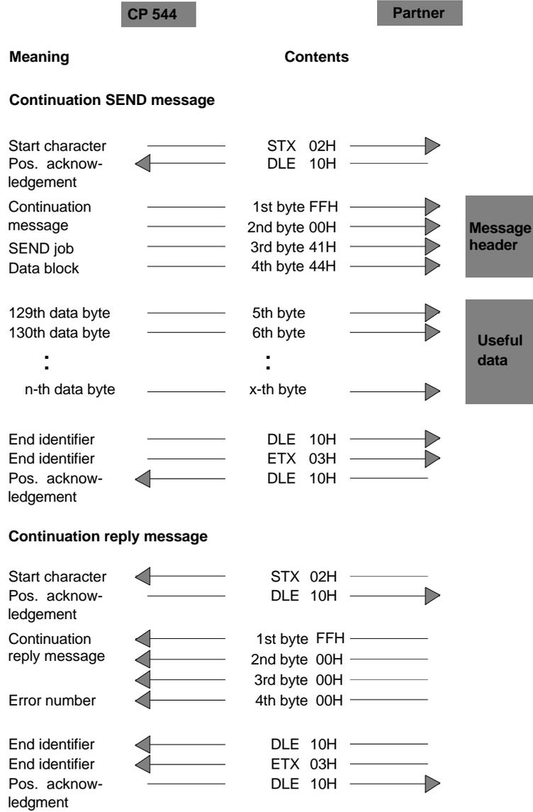
Fig. 3-11 Sequence of a continuation SEND message with continuation reply message
