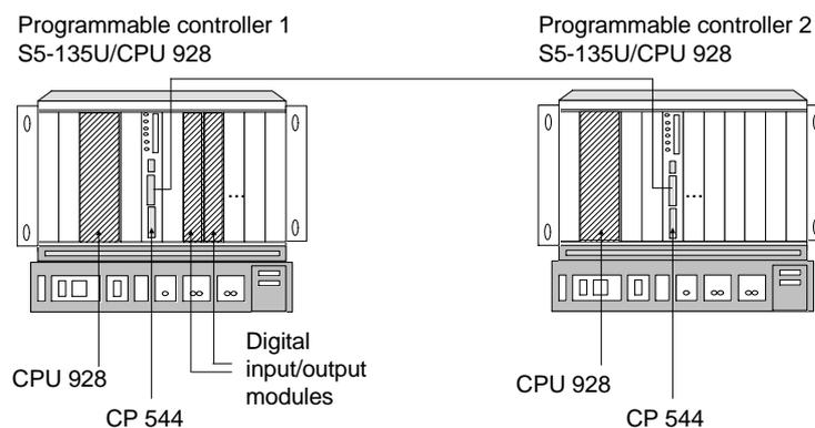
Fig. 9-1 System configuration in application example
