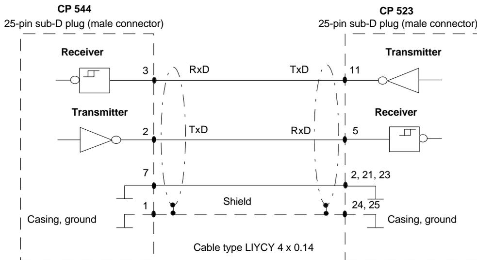
Fig. 10-11 V.24 submodule: connecting cable CP 544 - CP 523
