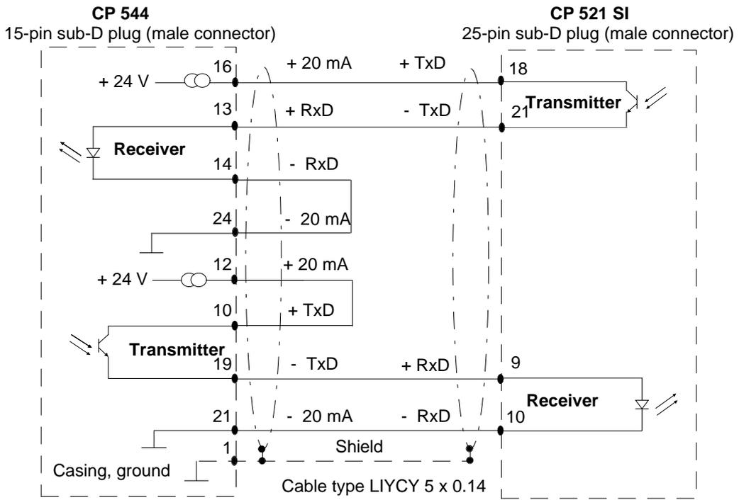
Fig. 10-7 TTY submodule: connecting cable CP 544 - CP 521 SI
