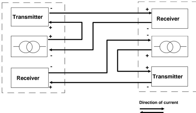
Fig. 1-4 TTY submodule: direction of loop current
