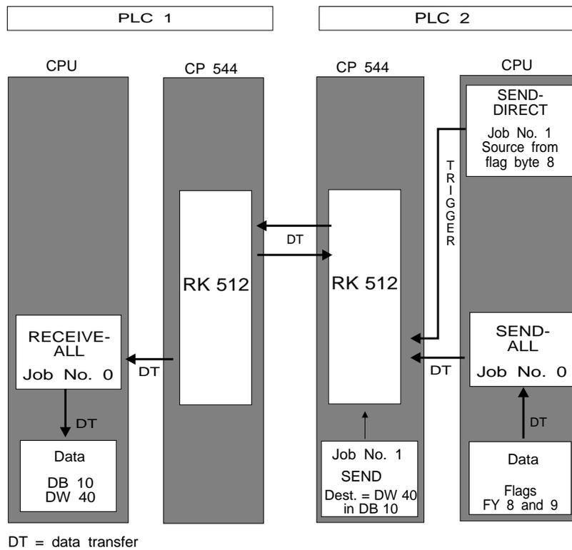
Fig. 9-5 Structure of a SEND job "Flag to DB"
