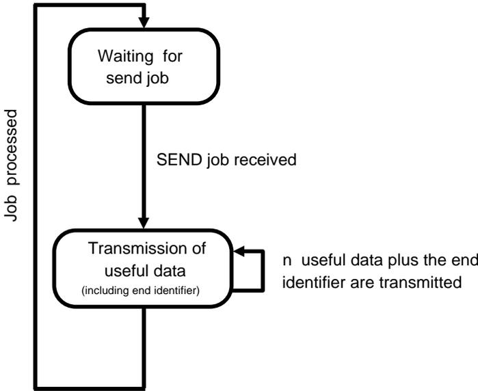
Fig. 5-6 Transmission sequence in mode 2
