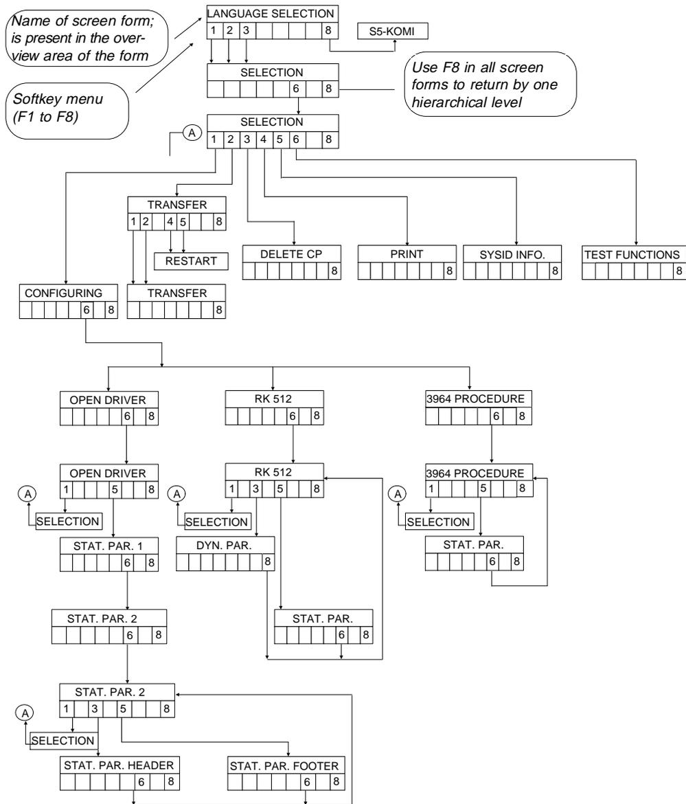
Fig. 7-1 Tree with screen forms of the COM PP parameter assignment software
