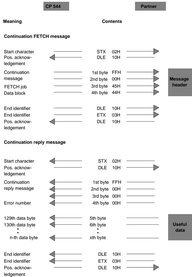
Fig. 3-14 Sequence of a continuation FETCH message with continuation reply message
