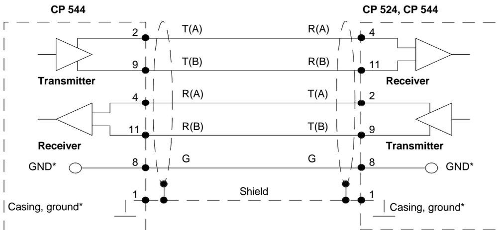
Fig. 10-2 RS422-A/485 submodule: connecting cable CP 544 - CP 524, CP 544
