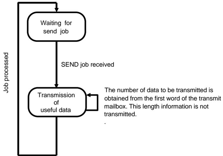
Fig. 5-4 Transmission sequence in mode 1
