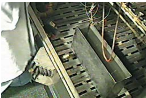
Finally immersed in water for 1 hour whilst energised at its rated voltage.
