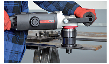
Steel plate beveling
