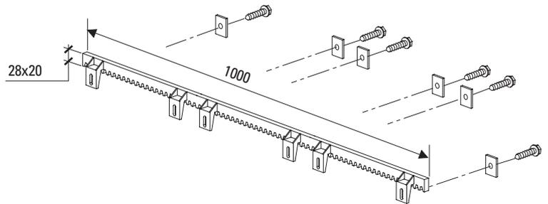
NYLON GEAR RACK 8 mm THICKNESS
