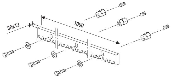
STEEL GEAR RACK WITH FIXING SLOTS
