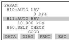
The lower range value is not changed, so the span changes. Parameter **C22** is changed at the same time.
