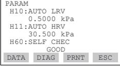
The higher range value is changed keeping the span constant.
