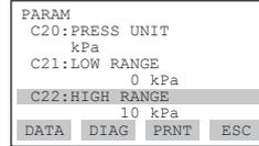
The low range value is not changed, so the span changes.
