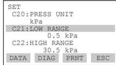
The higher range value is changed while the span remains constant.
