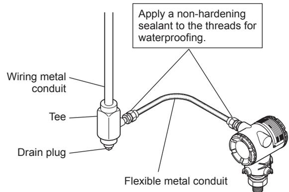
Figure 6.7 Typical Wiring Using Flexible Metal Conduit
