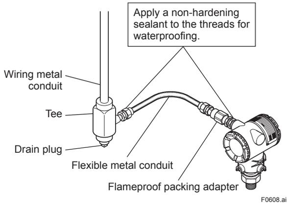
**Figure 6.8 Typical Cable Wiring Using Flameproof Packing Adapter**
