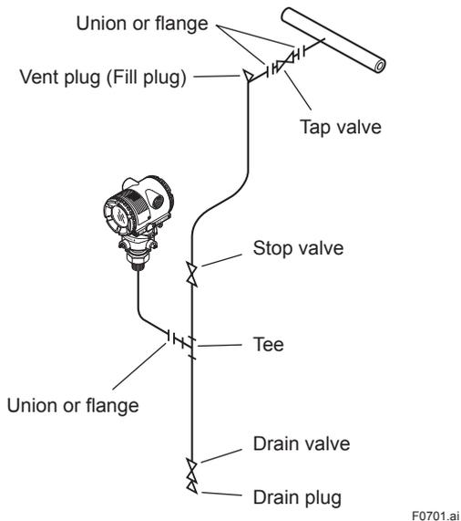
**Figure 7.1 Liquid Flow Measurement (Gauge Pressure Transmitters)**
